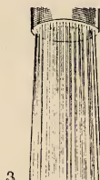
This liquid is forced through tiny holes of a spinnerette in fine streams. These are hardened into "filaments" or strands of rayon, which are woven into yarn.
