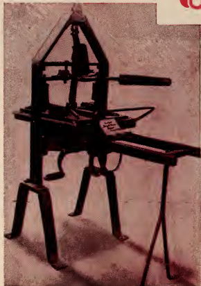
The hand-operated Ramage Press of pioneer days produced two papers a minute, provided an entire edition of 225 newspapers if no mishaps cropped up to vex the printer.
